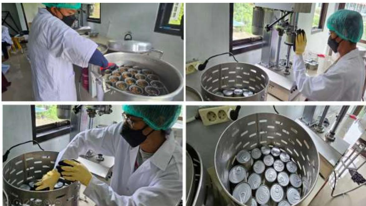
Figure 3. Exhausting Process, Can Closure and Sterilization of Canned Squid Sambel
